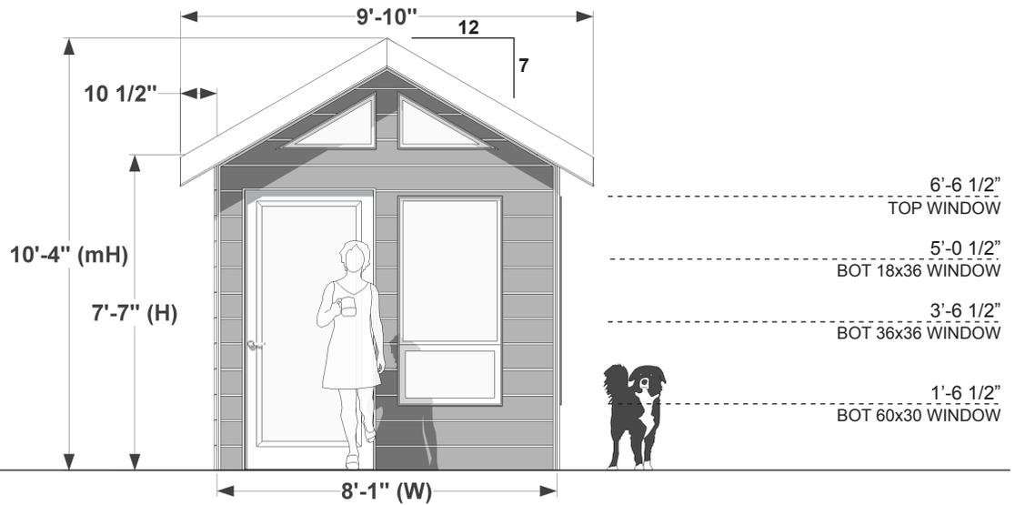
**(D)** = SHED DEPTH | **(W)** = SHED WIDTH | **(mH)** = MAX ROOF HEIGHT | **(H)** = SIDE WALL HEIGHT
